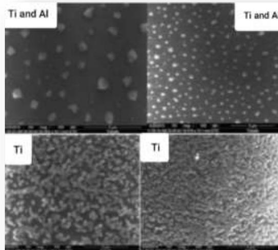
**Figure( 2) :** shows the image of membranes before and after the addition of aluminum through the SEM device
