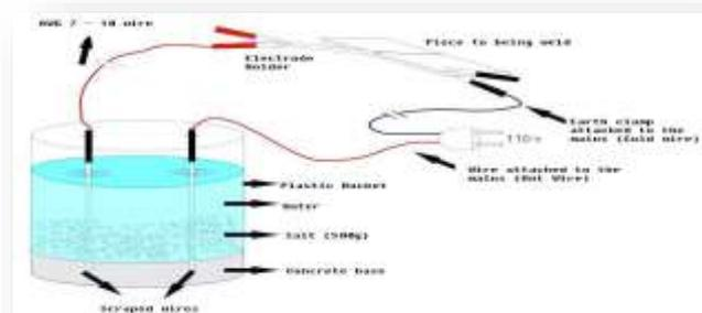
**Figure (1) :** shows direct welding method by using water
