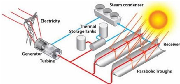
Fig. 4: Parabolic Trough CSP system
