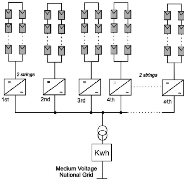
Fig. 8: Block diagram of the PV system
