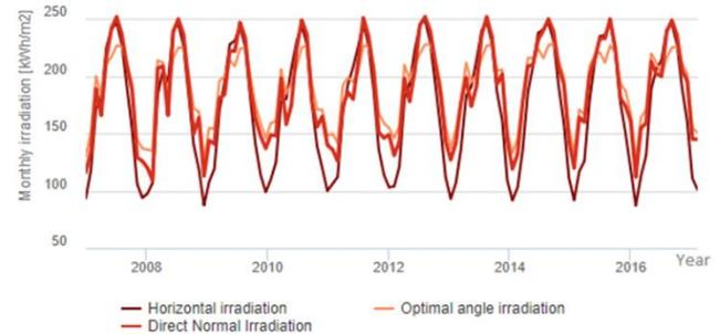
Fig. 1: Monthly solar irradiation at Brega selected site
